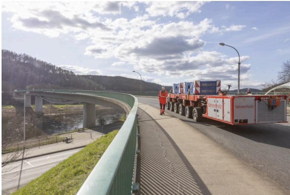
Figure 24 :The heavy-duty SPMT module with additional weights on the Elbe bridge in Bad Schandau (Stefan Gröschel)
